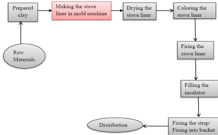
Figure 2: Semi-automation process of stove manufacturing
