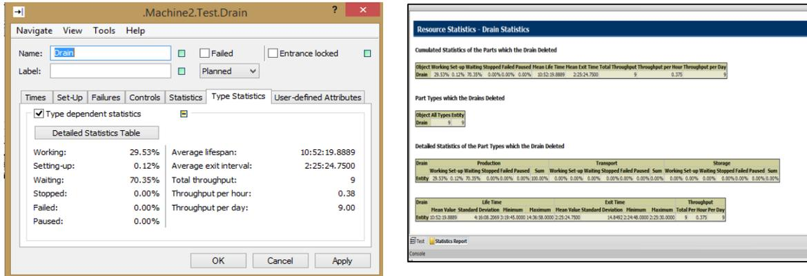
Figure 9: Result of semi automation production (machine 2)
