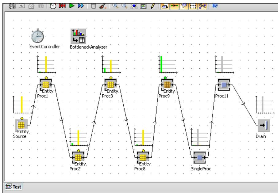
Figure 8: Process mapping of semi automation production (machine 2)
