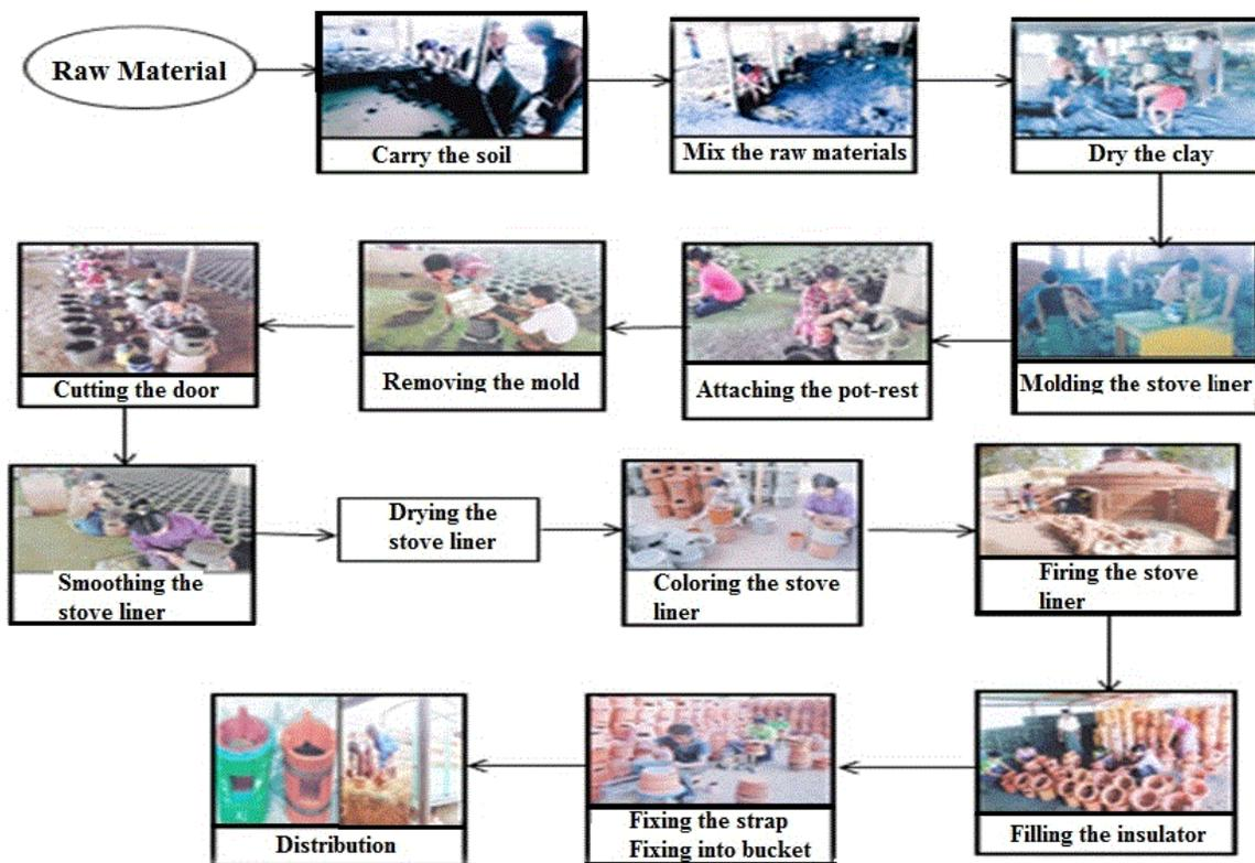
Figure 1: Current manual process of stove manufacturing
