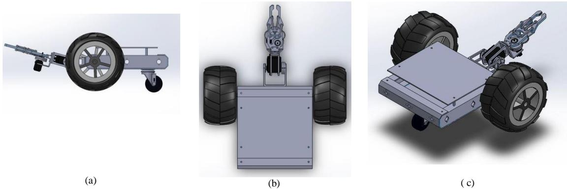
Fig. 2. CAD design of the robot: (a) Side view, (b) Top view, (c) Isometric view
