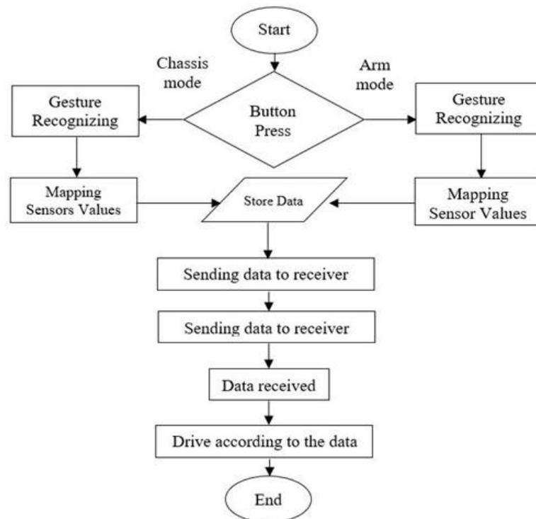
Fig 1. Overall process of controlling the robot system
