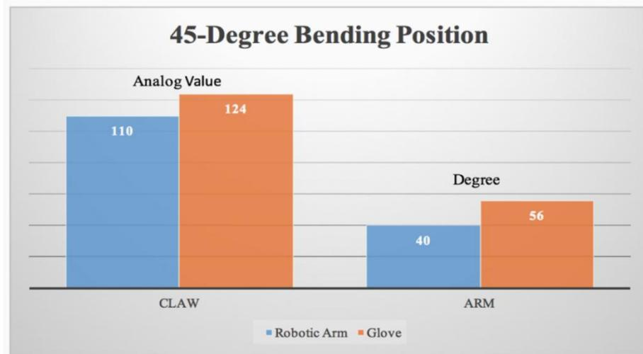
Fig. 12. Comparison between robotic arm and hand glove at 45-degree bending position
