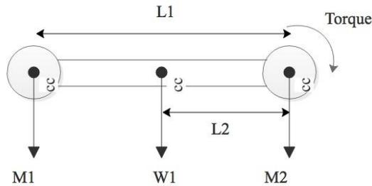
Fig. 7. Torque analysis in free body diagram
