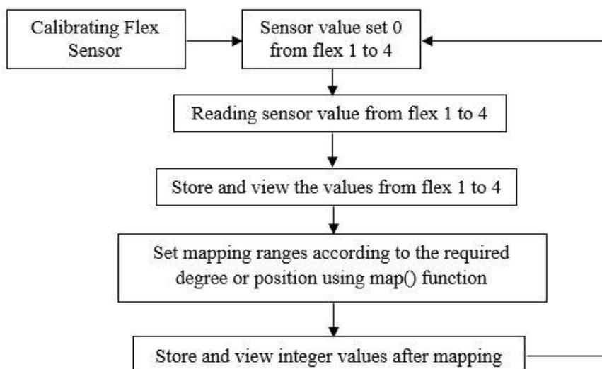
Fig. 5. Sensor Calibrating Process
