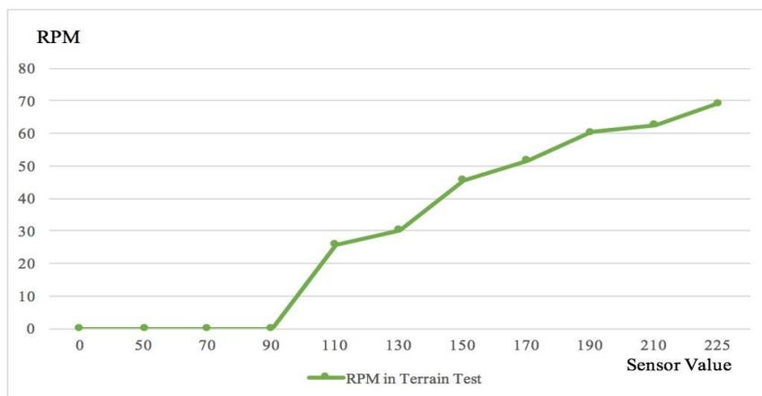
Fig. 10. RPM of DC motor during terrain test
