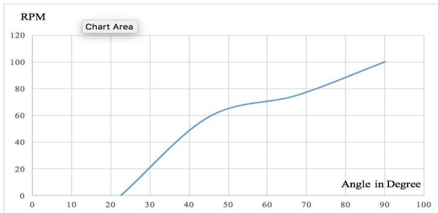
Fig. 9. RPM of DC motor vs angle of flex sensor
